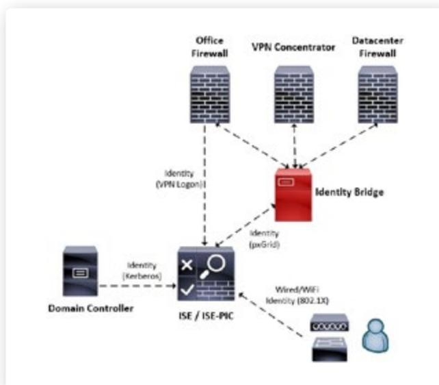
The Identity Bridge itself is a software component running on top of the Linux operating system with .NET support. The Identity Bridge communicates with Cisco ISE or Cisco ISE-PIC via the pxGrid 2.0 protocol. For this reason, it is important to have Cisco ISE or Cisco ISE-PIC version 2.3+ installed. The ASA image on the Cisco Secure firewall must be at least version 9.0+. Hardware requirements for Identity Bridge are minimal.
